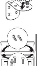
Move the door handles from the left to the right and cover the remaining holes with the hole cover pins.
